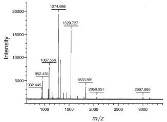
Figure 2. MALDI-TOF spectrum of a mixture of peptides obtained from tryptic digestion of hemoglobin (human).
