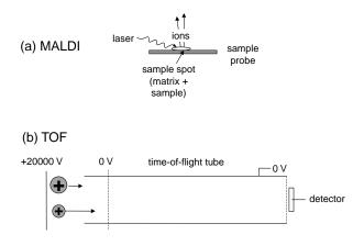
Figure 1. Schematic illustration of (a) MALDI and (b) TOF mass spectrometer. The potentials shown are provided solely as an example.
